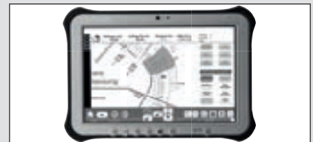
3D data on excavator computer
